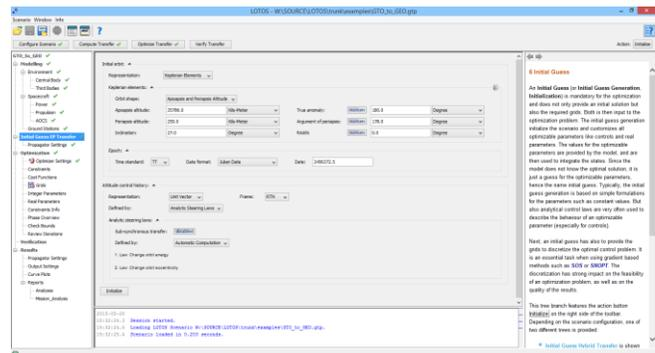
**Figure 2. Main window of the orbit transfer optimization and analysis software LOTOS. On the left the navigation tree is shown to access all configuration panels with one example shown in the center. Input is expected to define the whole scenario properties. The right panel shows content sensitive help to aid the user.**
