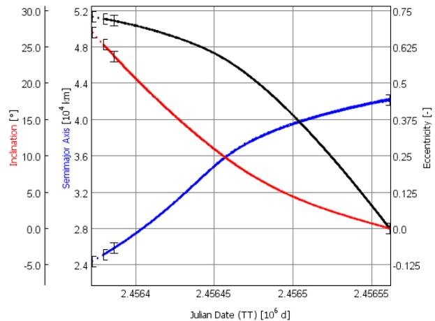
**Figure 7. Evolution of orbital elements semimajor axis (blue), eccentricity (black) and inclination (red) after re-optimization of the trajectory. The dotted lines at the beginning of the transfer indicate the already travelled part of trajectory (cycle #1). Directly next to it the second cycle can be identified within the symbols “[“ and “]”.**
