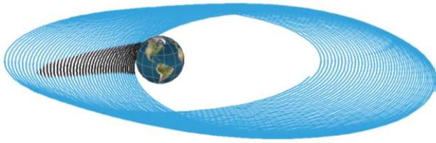
**Figure 5. Eclipses (black) during a multi-revolution low-thrust transfer (blue) illustrated in inertial frame.**
