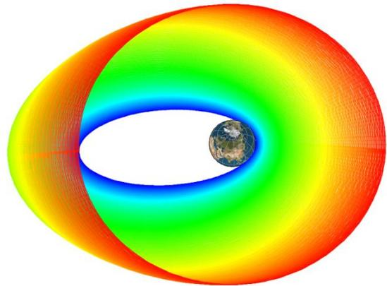
**Figure 1. Illustration of a typical low-thrust orbit transfer from GTO (blue) to GEO (red) lasting about 6 months. The top-down view shows more than 250 revolutions around the Earth.**
