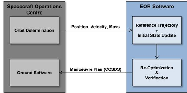
**Figure 6. One example of an operational chain for a ground-based navigation concept. The spacecraft operations center (left) is responsible for orbit determination and upload of the optimized maneuver plan to the spacecraft. The optimization software for the EOR scenarios handles the reference trajectory and its re-optimization considering the updated spacecraft states.**
