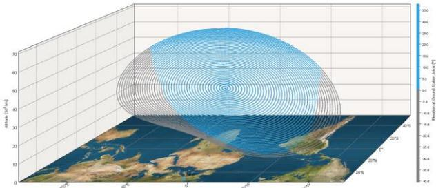
**Figure 3. Synchronous orbit transfer (grey) to GEO with ground station in Stuttgart, Germany, and its visibility from the spacecraft (blue). The south-north map illustrates how an observer at the ground station actually “sees” the spacecraft trajectory.**
