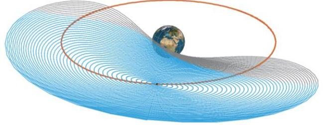
**Figure 4. Synchronous orbit transfer (grey) in Earth-rotating frame with ground station visibility (blue) and GEO ring (brown).**
