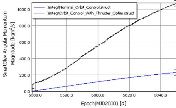
Figure 3. Impact of thruster orientation optimisation on angular momentum vector magnitude
