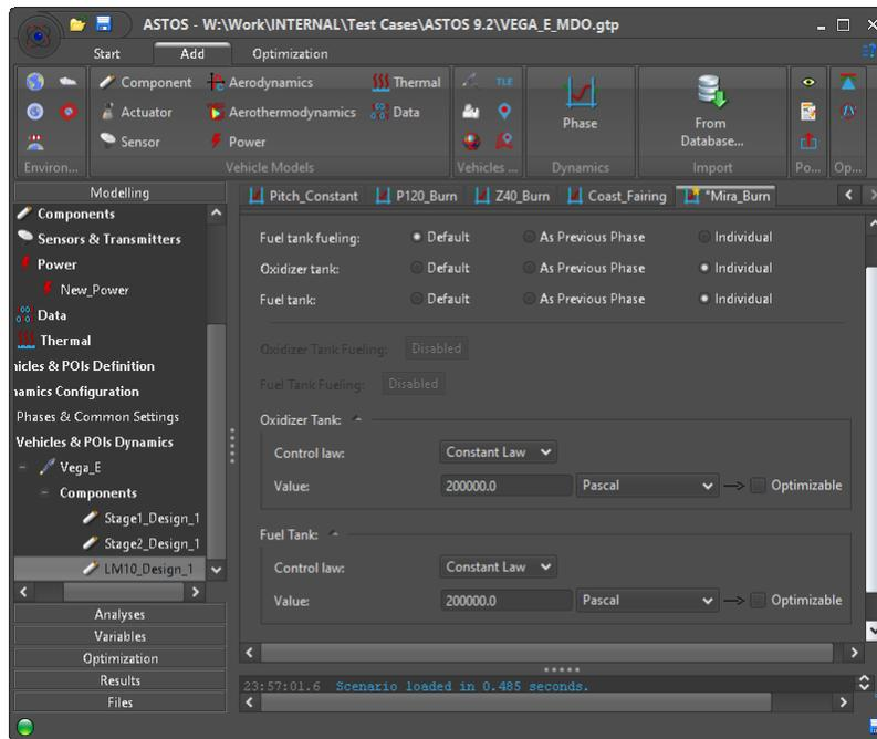
**Fig. 4 Phase-specific definition of tank pressure.**
